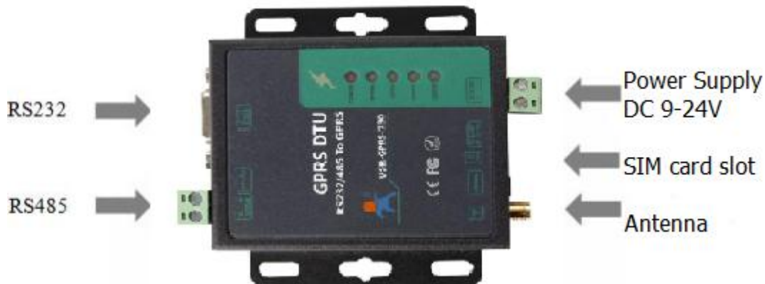
Figure 5 hardware interface schematic diagram
