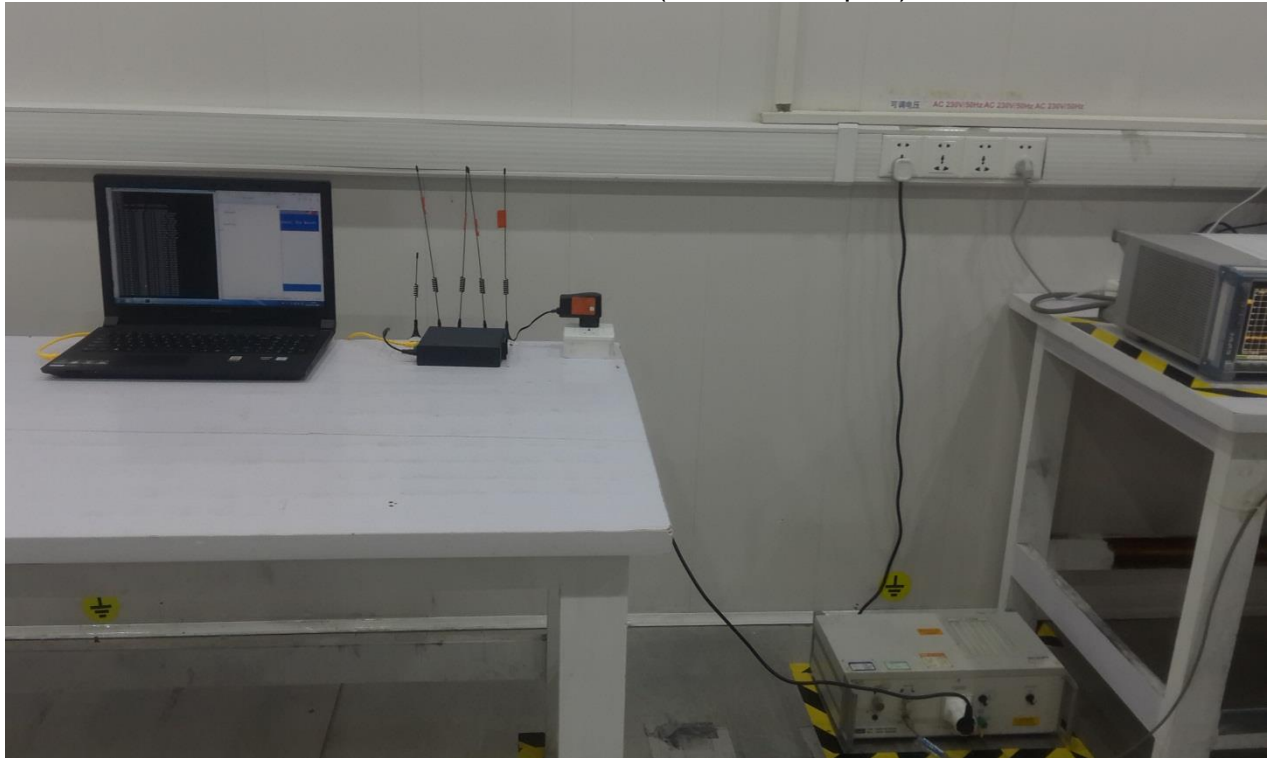
Conducted Emission(for AC main port)
