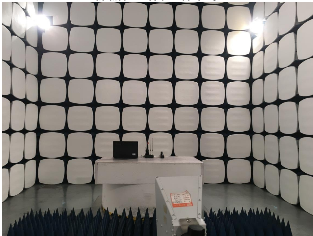
Radiated Emission Above 1GHz
