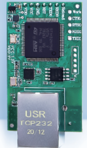
USR-TCP232-E2 Dual UART PIN Ethernet Module
